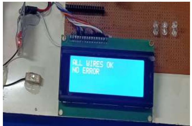
Figure 9: LCD Displaying No Fault
