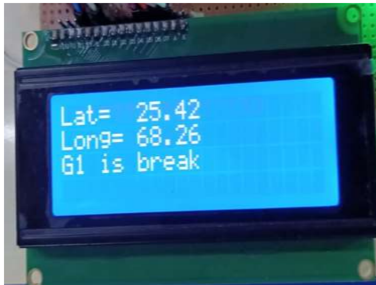
Figure 11: LCD displaying Fault and Location
